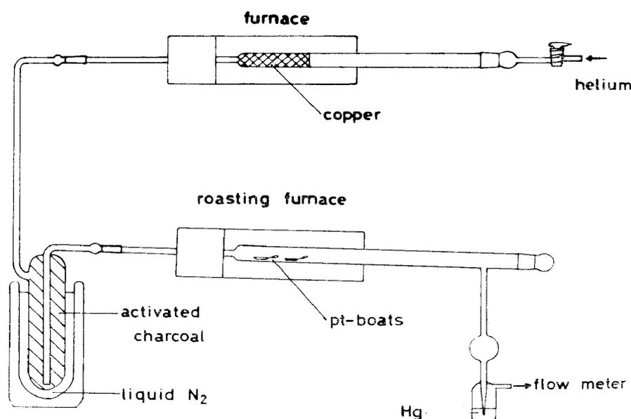
Fig. 10. Carbonate roasting system.
