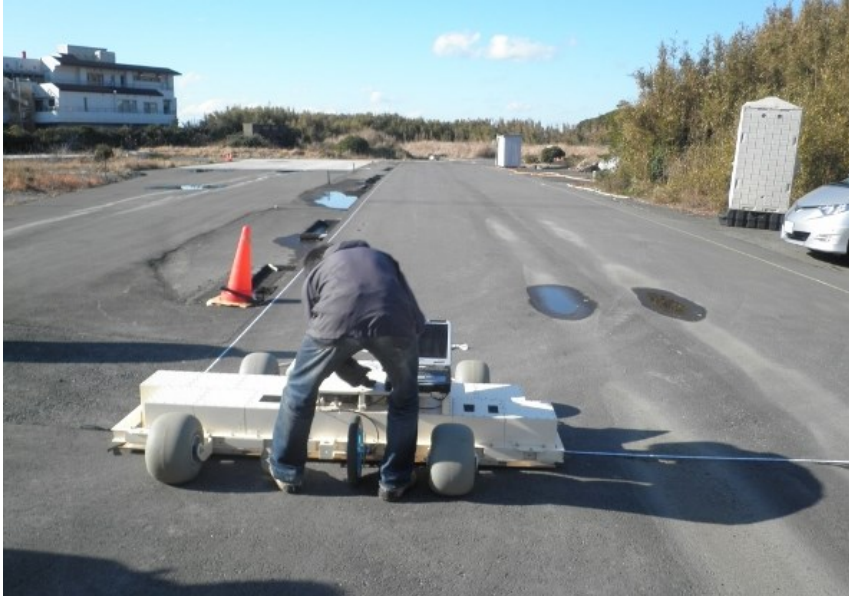
Figure 7.12 Data acquisition with YAKUMO on the airport runway model in Nobi experiment site.
