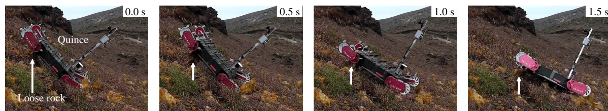
Figure 1. Tracked robot "Quince" sliding down owing to rolling of loose rocks at Mt. Aso
