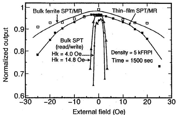
Fig. 5 Influence of external field for various single pole heads with a double-layered medium.
