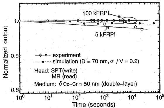
Fig. 2 Dependence of time decay upon recording density.
