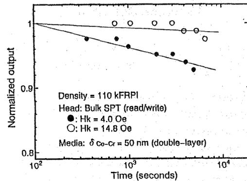
Fig. 3 Dependence of time decay upon main pole anisotropy field  $H_k$ .
