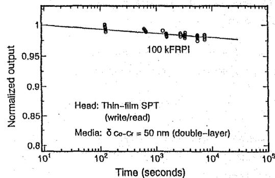
Fig. 4 Time decay of output with thin-film return path head.
