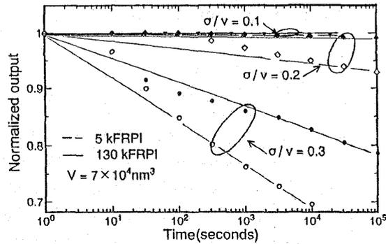
Fig. 1 Time decay at various recording densities and volume deviations.
