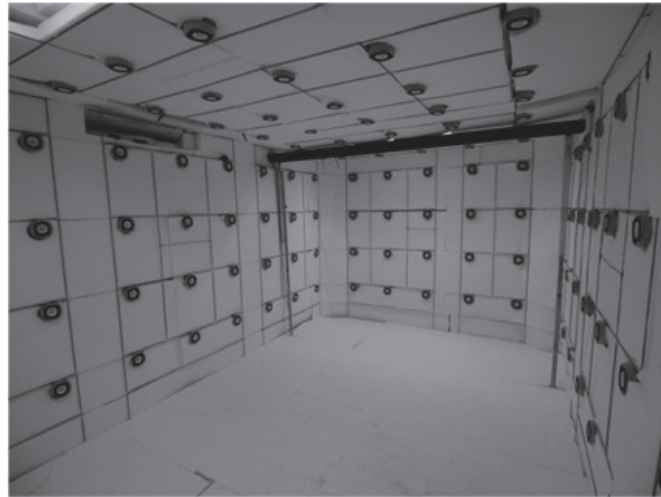
(b) The 157-channel irregular loudspeaker array built inside an anechoic chamber
