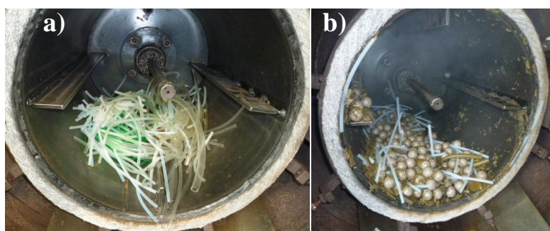
Figure 4. Mixture of plastic tubes a) before and b) after processing in Johnson boiler-ball mill. FPVC tubes are originally transparent and PE tubes are white and green.
