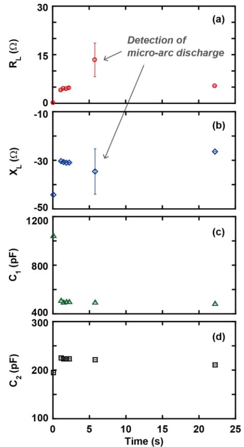
Fig. 4 Time variations of (a) real part of load impedance  $R_L$ , (b) imaginary part of load impedance  $X_L$ , (c) capacitance of variable capacitor  $C_1$ , (d) capacitance of variable capacitor  $C_2$ .
