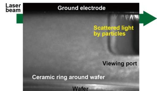
Fig. 3 Image of laser light scattered by particles.
