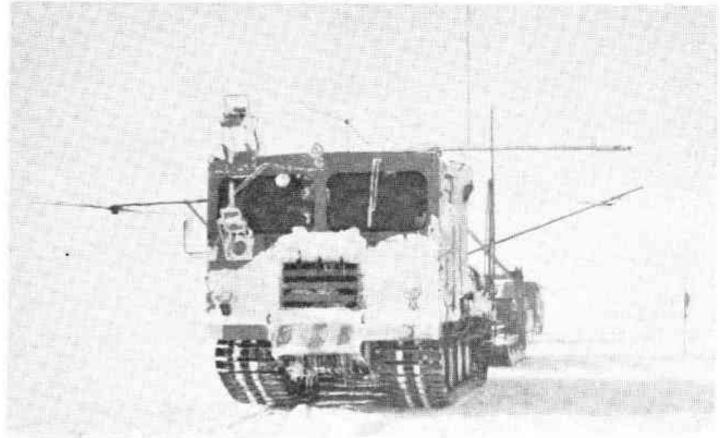
Fig. 2 KD608 snow-car, Radio echo sounding an- tennas are fixed on both sides of snow-car.
