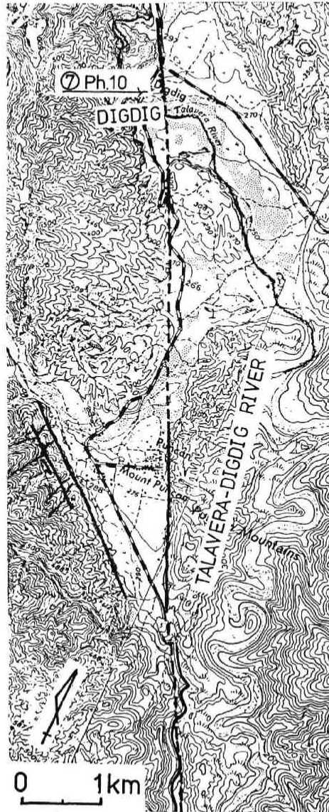
Fig. 7 Fault traces along the Talavera-Digdig River
