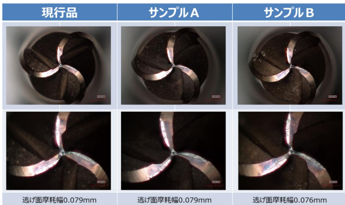
Fig.6-8 Wear amount at the cutting distance of 30m.
