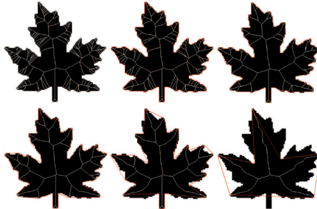
Figure 2.9: Distance field based method and its pruning step proposed in [35]
