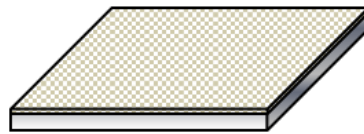
2. Anode formation (Graphene)
