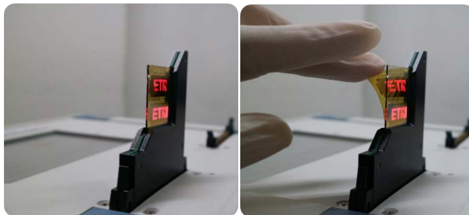
Figure 5.7. Flexible OLED with pixelated graphene films as transparent electrodes.
