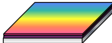
4. Organics deposition (HTL/EML/ETL)
