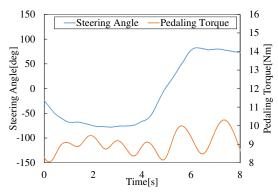
Fig. 16: Pedaling torque with proposed method
