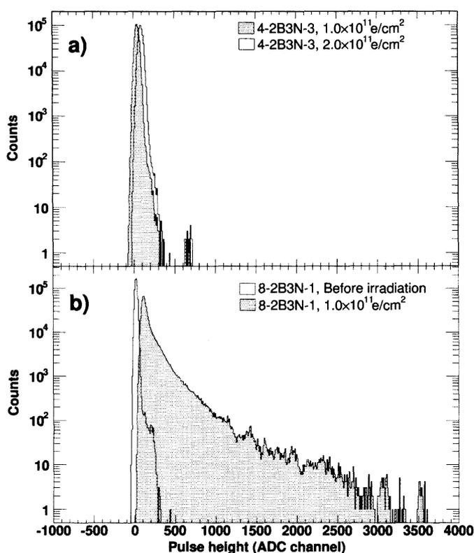
Fig.2. Distribution of dark current of CCDs (a) after irradiation of  $1 \times 10^{11}/\text{cm}^2$  and  $2 \times 10^{11}/\text{cm}^2$   $\beta$  ray of  $^{90}\text{Sr}$  and (b) before and after  $1 \times 10^{11}/\text{cm}^2$  140 MeV electron beam irradiation [8].
