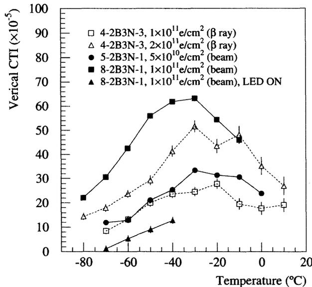
Fig.3. Charge transfer inefficiency (CTI) as a function of temperature. CTI with fat-zero charge injection of  $\sim 1200$  electrons/pixel is also plotted [8].
