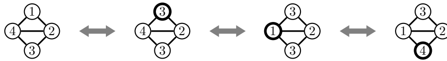
Figure 1.2: A transformation of 4-colorings. A vertex which is recolored from the previous 4-coloring is depicted by a thick circle.
