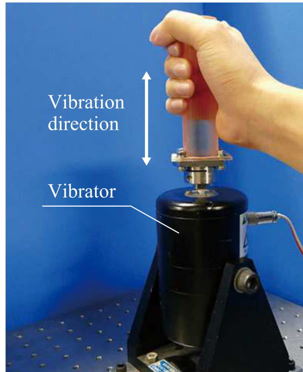
Figure 2.9: (a) Participant perceiving vibrotactile stimulation generated by a vibrator
