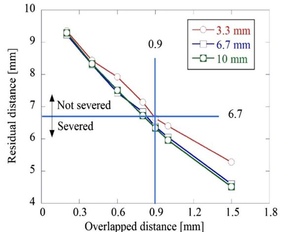
Fig. 5 Residual distance of tether (diameter of tether is 10 mm).
