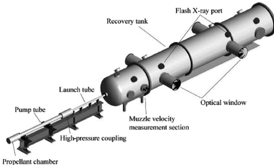
Fig. 8 Illustration of high-explosive gun used in hypervelocity impact experiment.
