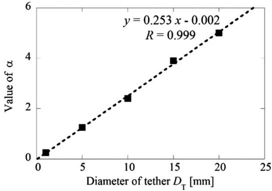
Fig. 6 Fracture progress  $\alpha$  for diameter of tether  $D_T$ .
