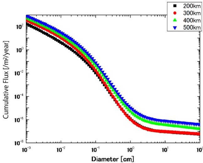
Fig. 12 Debris flux determined from ORDEM model provided by NASA.
