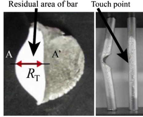
**Fig. 10** Aluminum bars after impact.
