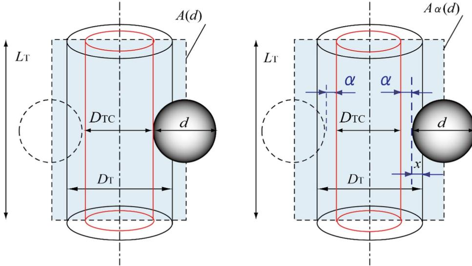
Fig. 11 Effective cross-sectional area (left: conventional approach, right: proposed approach).
