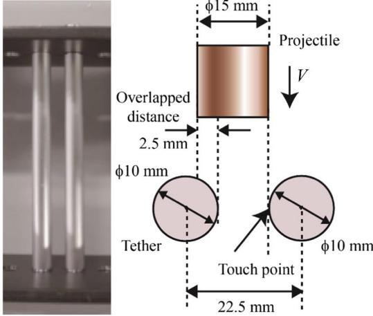
**Fig. 9** Target bars for impact experiments (left end of right bar is touch point).
