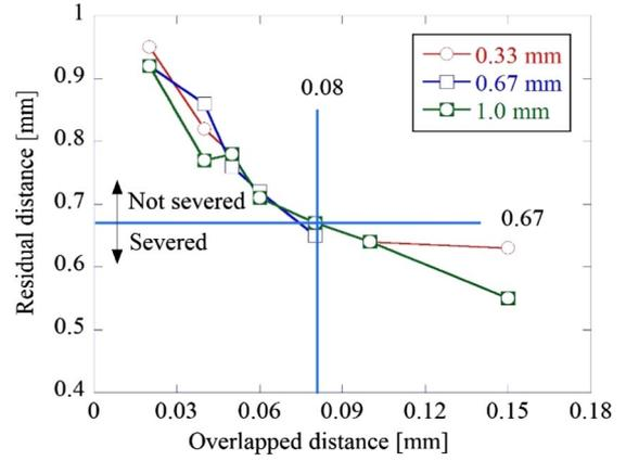
Fig. 4 Residual distance of tether (diameter of tether is 1.0 mm).
