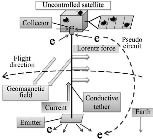
4 Fig. 1 Principle of electrodynamic tether.
