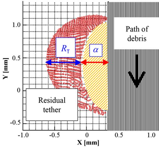
Fig. 3 Cross section of tether after collision ( $V = 6.0$  km/s and  $d = 1$  mm).
