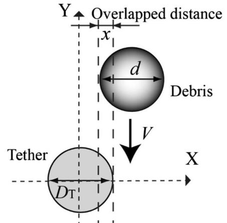
Fig. 2 Initial positions of debris and tether before collision in numerical simulation model.
