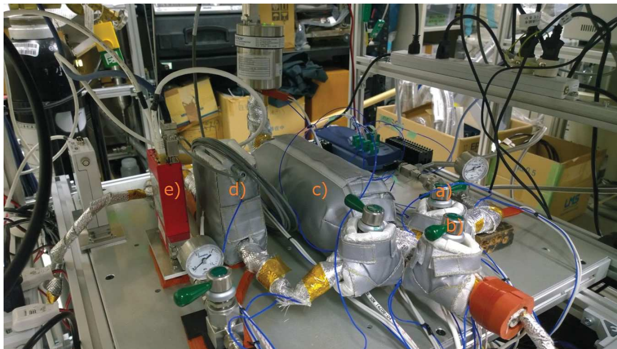
Figure 2.A.2: Heated mixing tank. a) Valve for N_2 and vacuum pump. b) Inlet for liquid fuel. c) Heated mixing tank. d) Mass flow controller for fuel/ N_2 mixture. e) Mass flow controller for O_2 .
