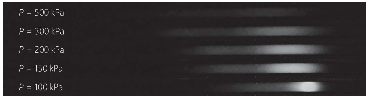
Figure 4.3.3: Weak flame images of iso -octane for a dilution ratio of 20% CO 2 at \Phi = 1.0 and pressures between 100 kPa and 500 kPa.
