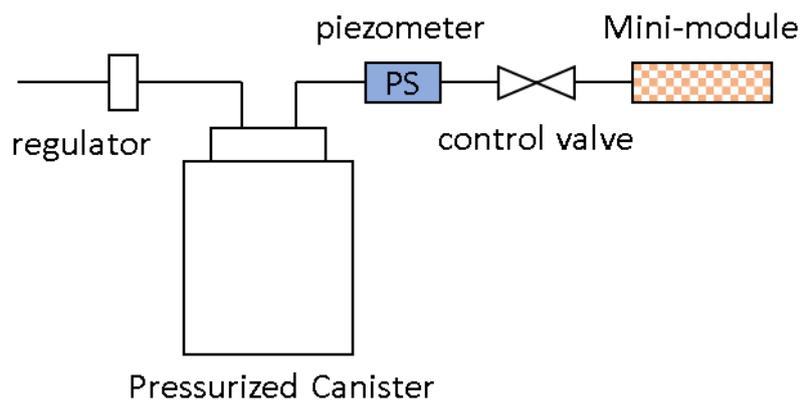
**Fig. 3.4 Mini-module cleaning equipment.**
