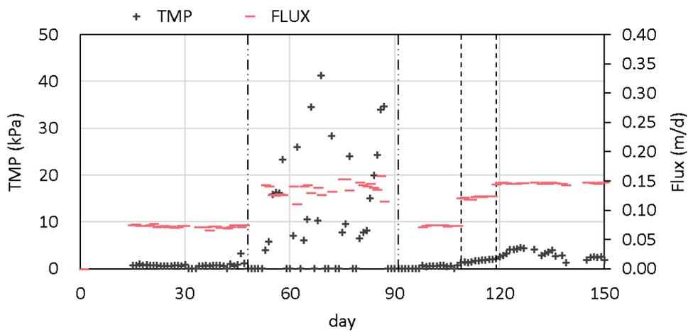
**Fig. 3.9 TMP – FLUX record during the long-term operation.**
