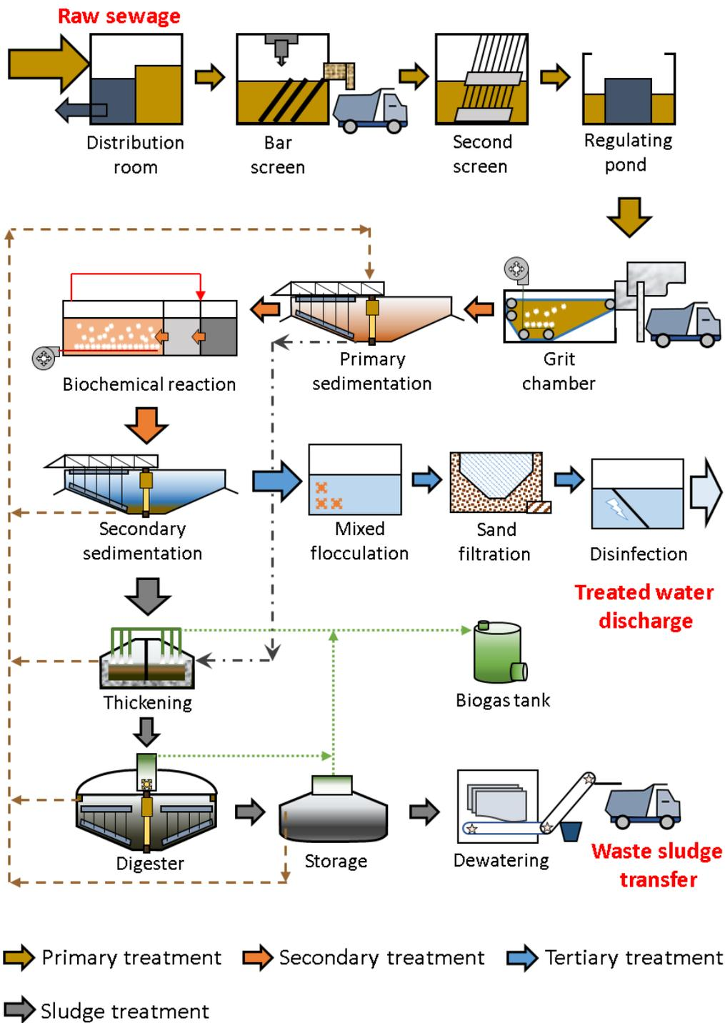
**Fig. 2.1 A typical sewage treatment process in WWTP.**
