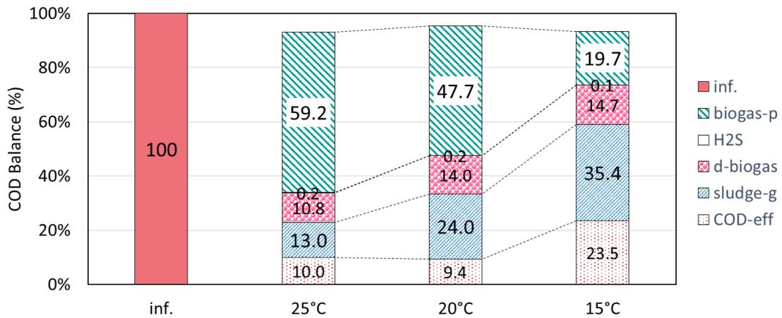
**Fig. 5.11 COD balance in different temperatures (%).**
