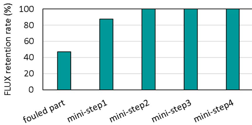
**Fig. 3.22 Mini membrane module cleaning result.**
