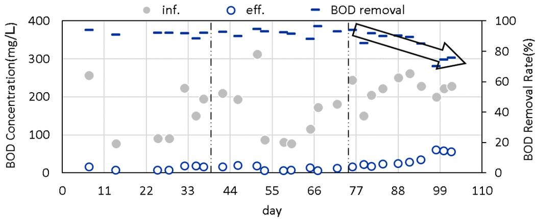
**Fig. 5.2 BOD in influent and effluent and the removal efficiency.**
