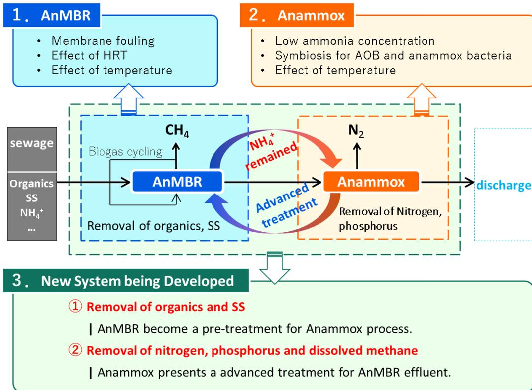
Fig. 2.10 Combined process by AnMBR and anammox process.
