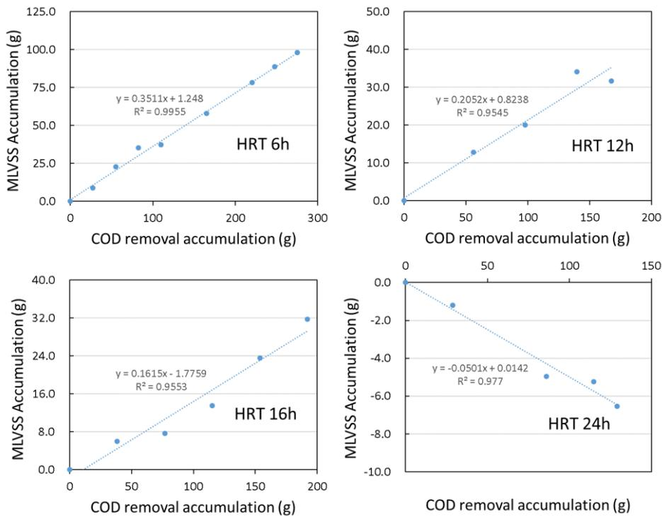
**Fig. 5.22 Sludge yield calculation in different condition.**
