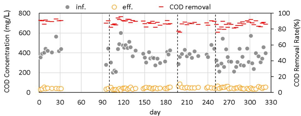
**Fig. 4.1 COD in influent and effluent and removal efficiency during long-term operation.**
