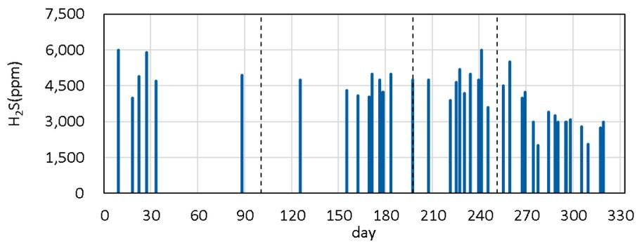
**Fig. 4.9 H<sub>2</sub>S gas produced during long-term operation.**
