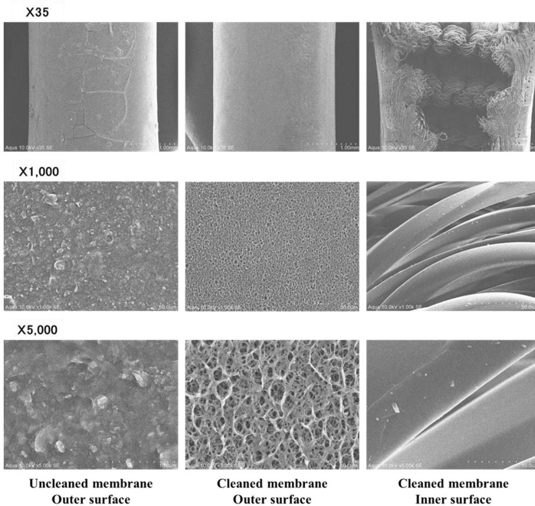
**Fig. 3.23 SEM results of outer membrane surface as before and after cleaning.**
