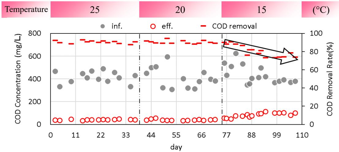
**Fig. 5.1 COD in influent and effluent and the removal efficiency.**
