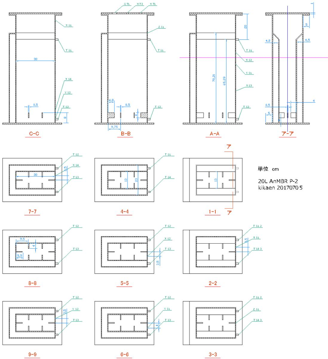
**Fig. A.2 Details of the New-designed AnMBR transversal drawing.**
