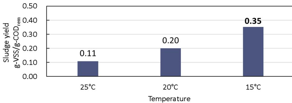
**Fig. 5.7 Sludge yield in different temperature conditions.**
