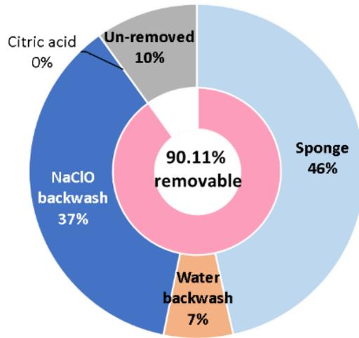
**Fig. 3.20 Fouled removable analysis via membrane off-line cleaning.**
