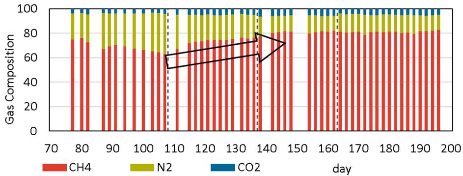
**Fig. 5.25 Biogas composition during the long-term operation.**
