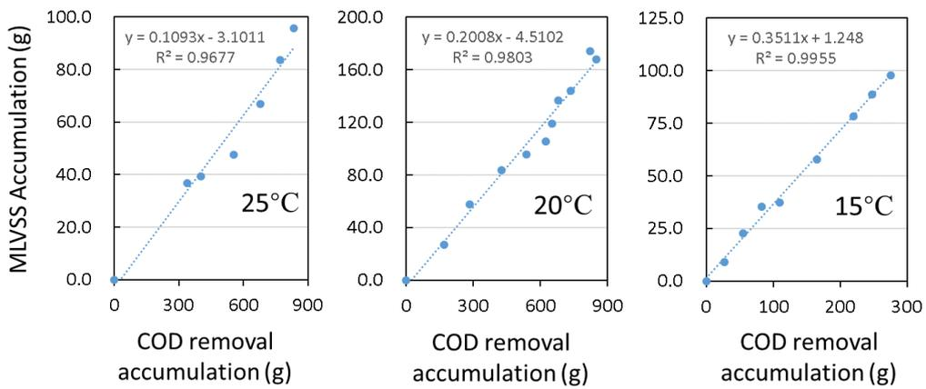
**Fig. 5.6 Sludge yield calculation in each temperature condition.**
