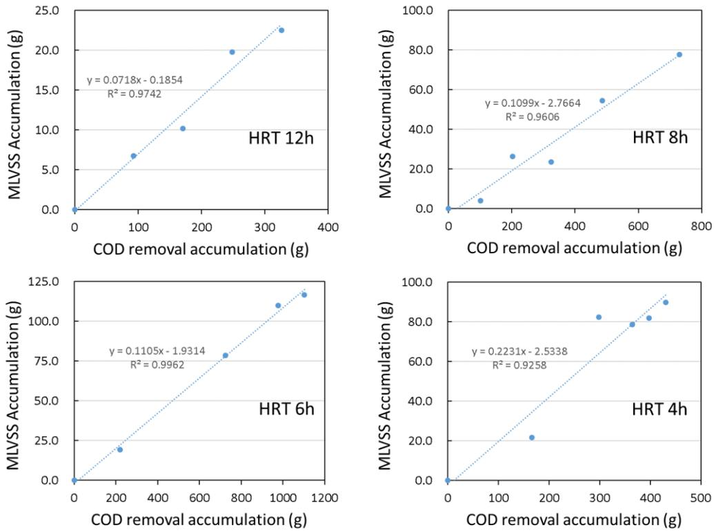
**Fig. 4.5 MLSS accumulation by the COD<sub>rem</sub> accumulation in each HRT.**
