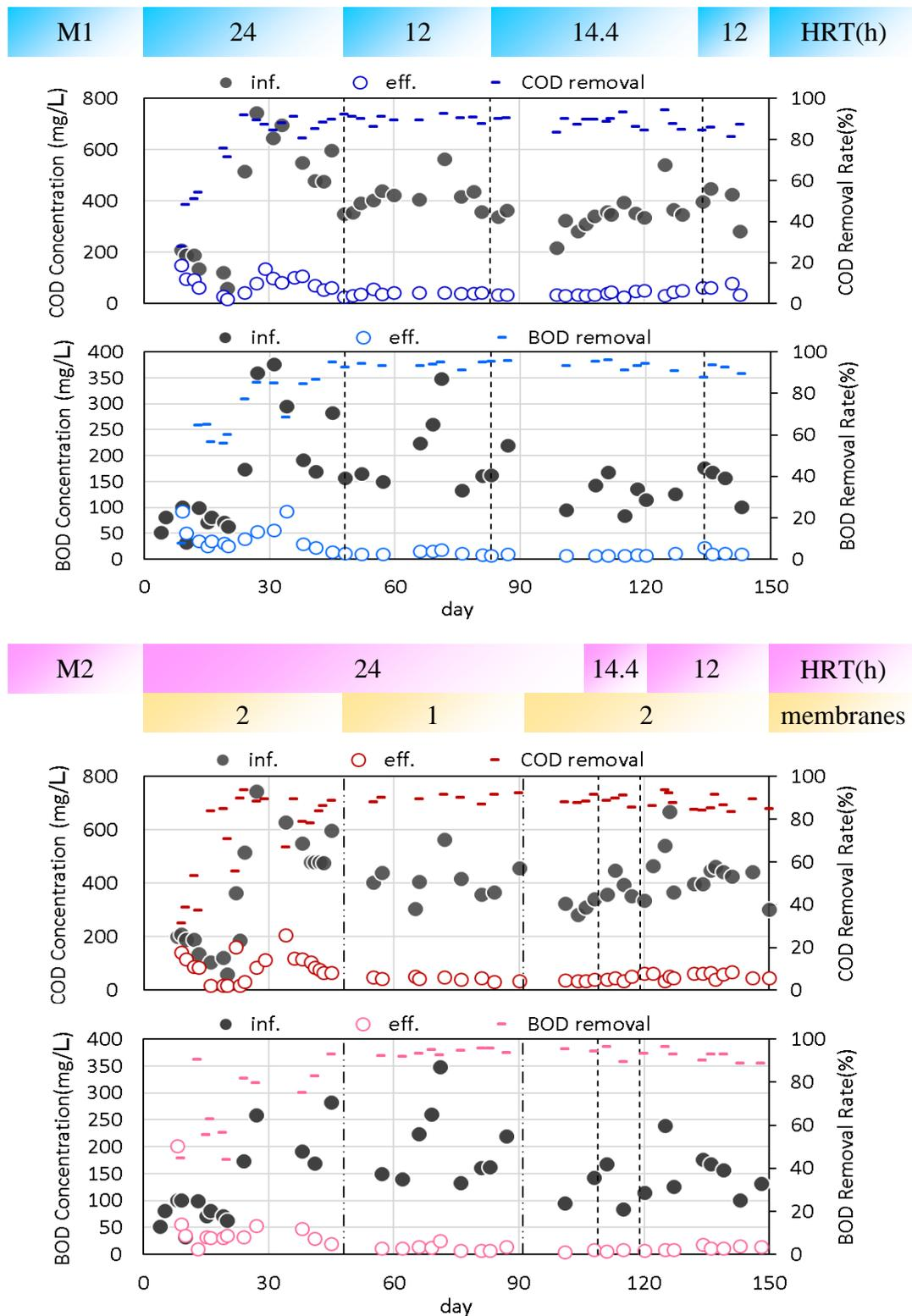
**Fig. 3.6 COD and BOD of influent and effluent and the removal efficiency.**
