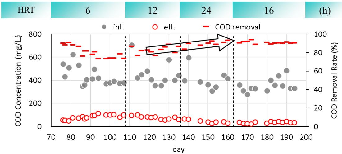
**Fig. 5.17 COD in influent and effluent and the removal efficiency.**
