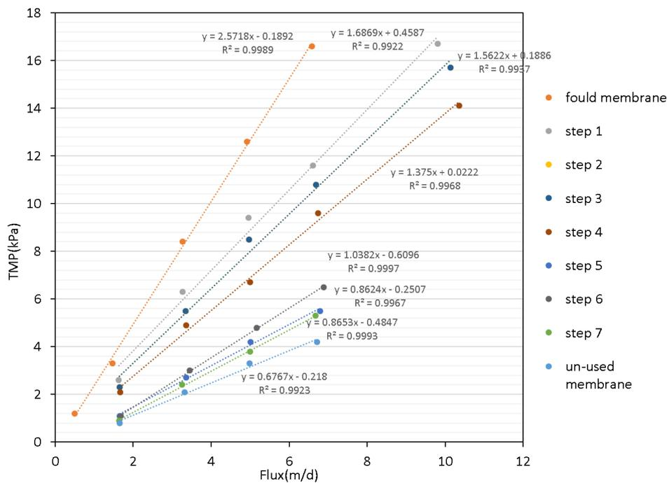
**Fig. 3.19 Original TMP-FLUX data of off-line cleaning.**
