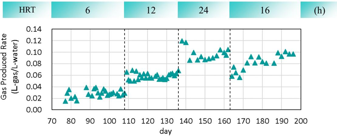
**Fig. 5.24 Biogas production rate during the long-term operation.**
