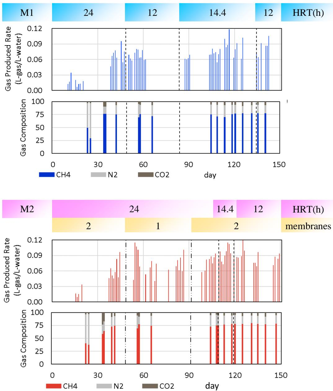
**Fig. 3.7 Biogas production rate and the composition.**
