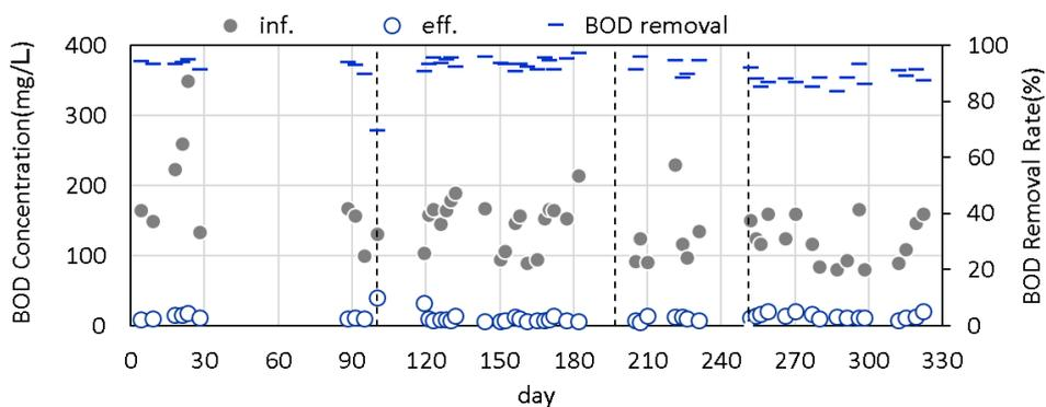
**Fig. 4.2 BOD in influent and effluent and removal efficiency during long-term operation.**
