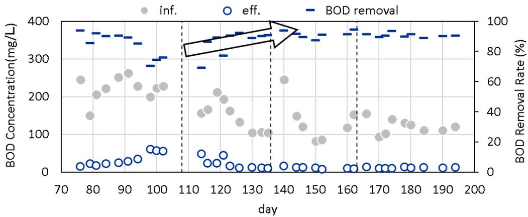
**Fig. 5.18 BOD in influent and effluent and the removal efficiency.**
