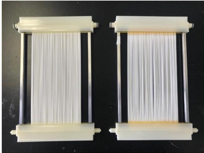
**Fig. 3.1** Two kinds of membrane (pore size, left:0.4 $\mu$ m; right0.05 $\mu$ m).
