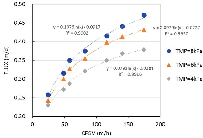
**Fig. 3.11 The relations between FLUX and CFGV.**
