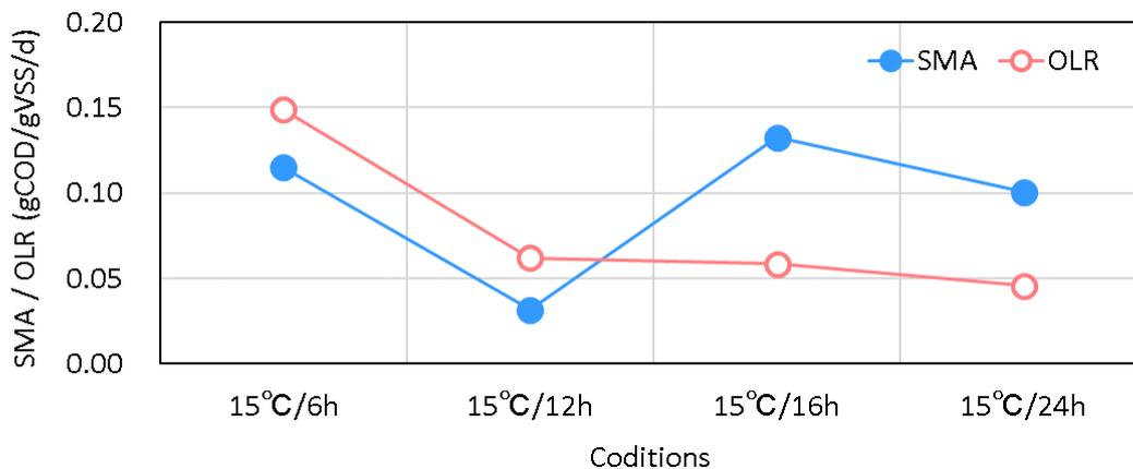
**Fig. 5.28 SMA&OLR in different HRTs at low temperature operation.**
