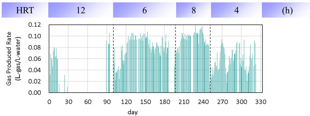
**Fig. 4.7 Biogas production rate during long-term operation.**
