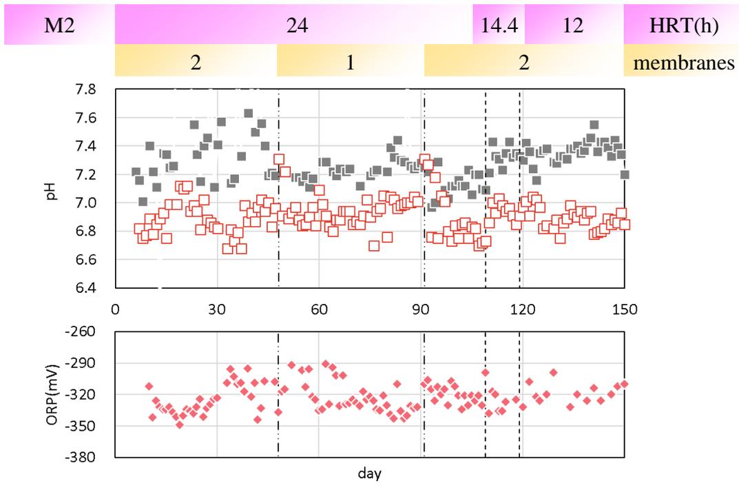
**Fig. 3.14** Influent and effluent pH and ORP in AnMBRs.
