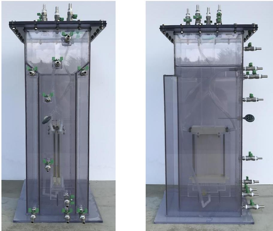
**Fig. A.4 Photographs of the New-designed AnMBR with membrane module.**
