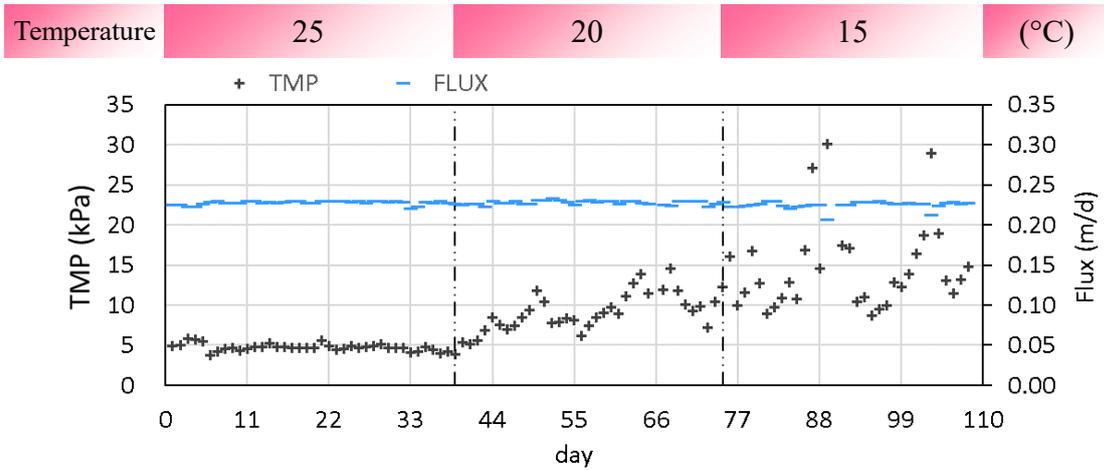
**Fig. 5.13 TMP – FLUX record during the long-term operation.**
