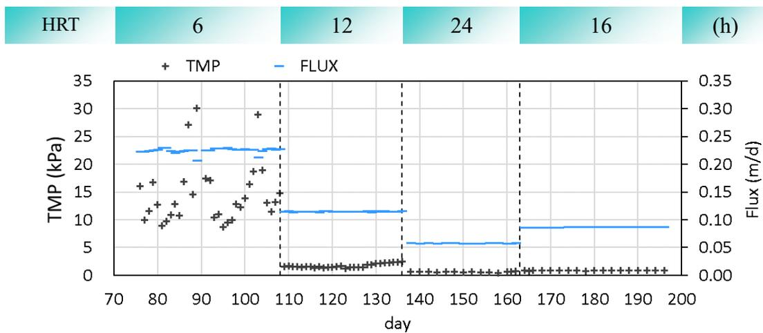
**Fig. 5.29 TMP – FLUX record during the long-term operation.**
