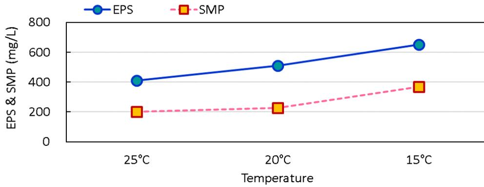
**Fig. 5.15 EPS and SMP in different temperature conditions.**
