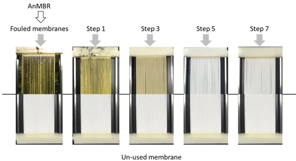
**Fig. 3.18 Photographs taken after off-line membrane cleaning steps.**
