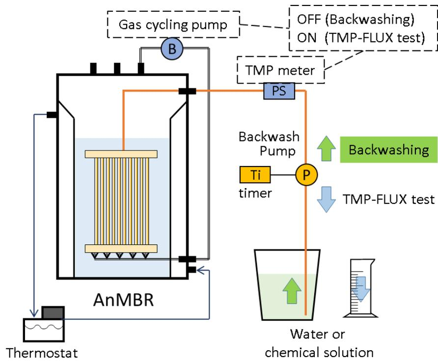
**Fig. 3.3 Off-line membrane cleaning equipment.**
