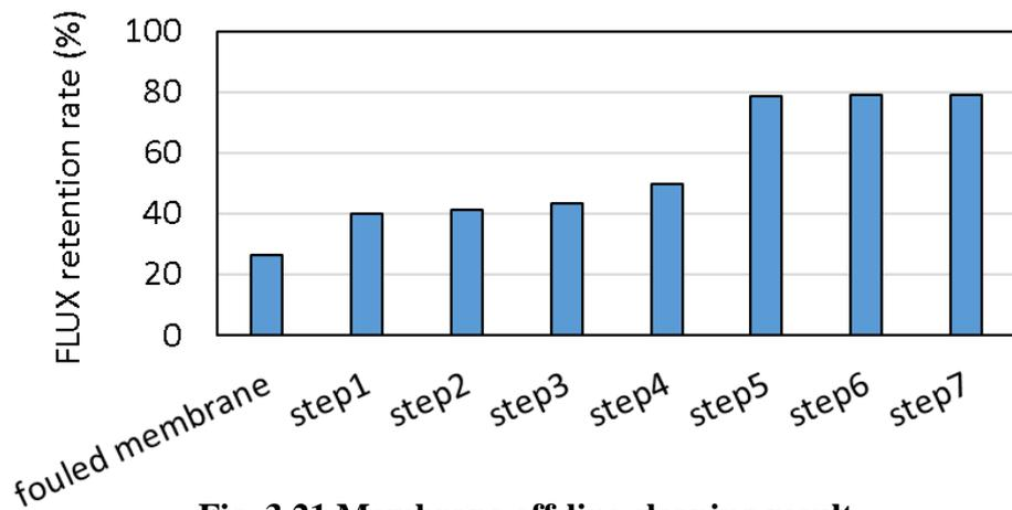
**Fig. 3.21 Membrane off-line cleaning result.**
