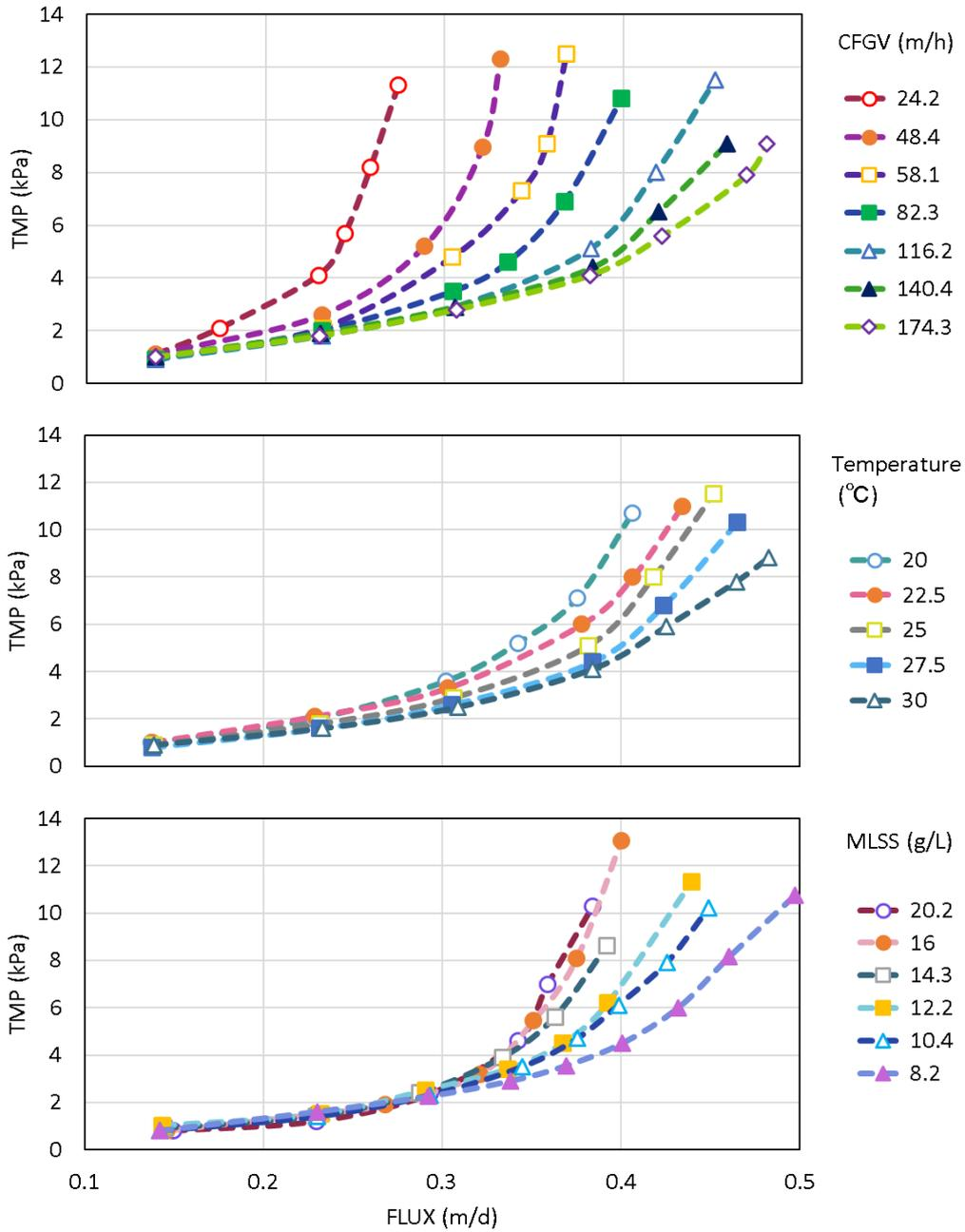
**Fig. 3.10 TMP - FLUX tests in different CFGV, temperature and MLSS conditions.**
