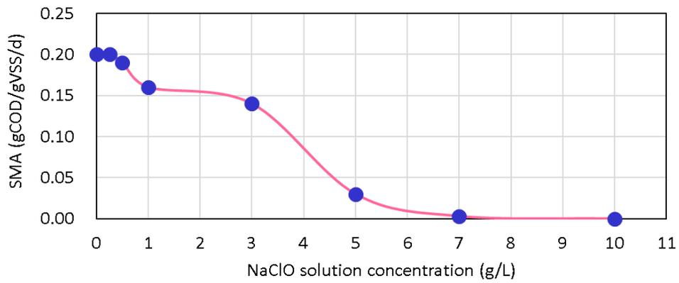
**Fig.3.17** Specific methanogenic activity in different NaClO solution.
