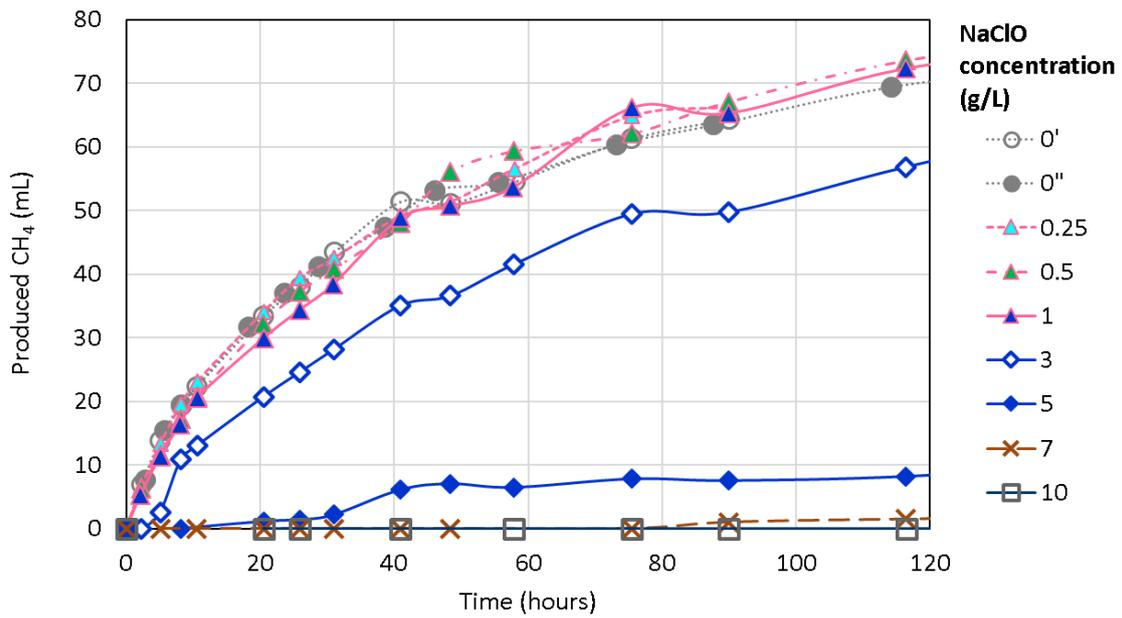
**Fig. 3.16** Methane gas produced during the activity test.
