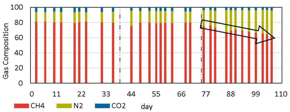
**Fig. 5.9 Biogas composition during the long-term operation.**
