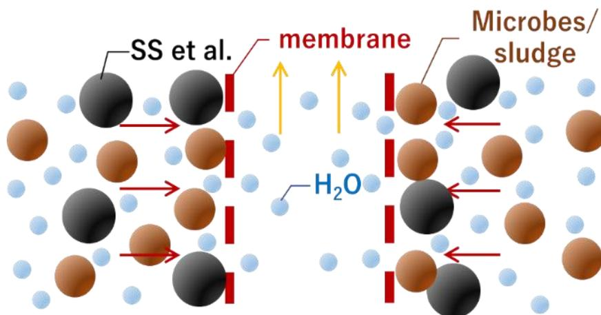
**Fig. 2.2 Membrane filtration principle.**
