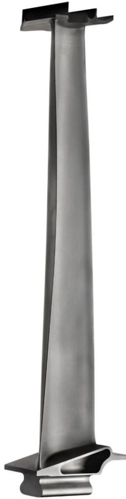
Fig. 1.6. PBF-EB-built Low-Pressure Turbine blade in  $\gamma$ -titanium aluminide [56].
