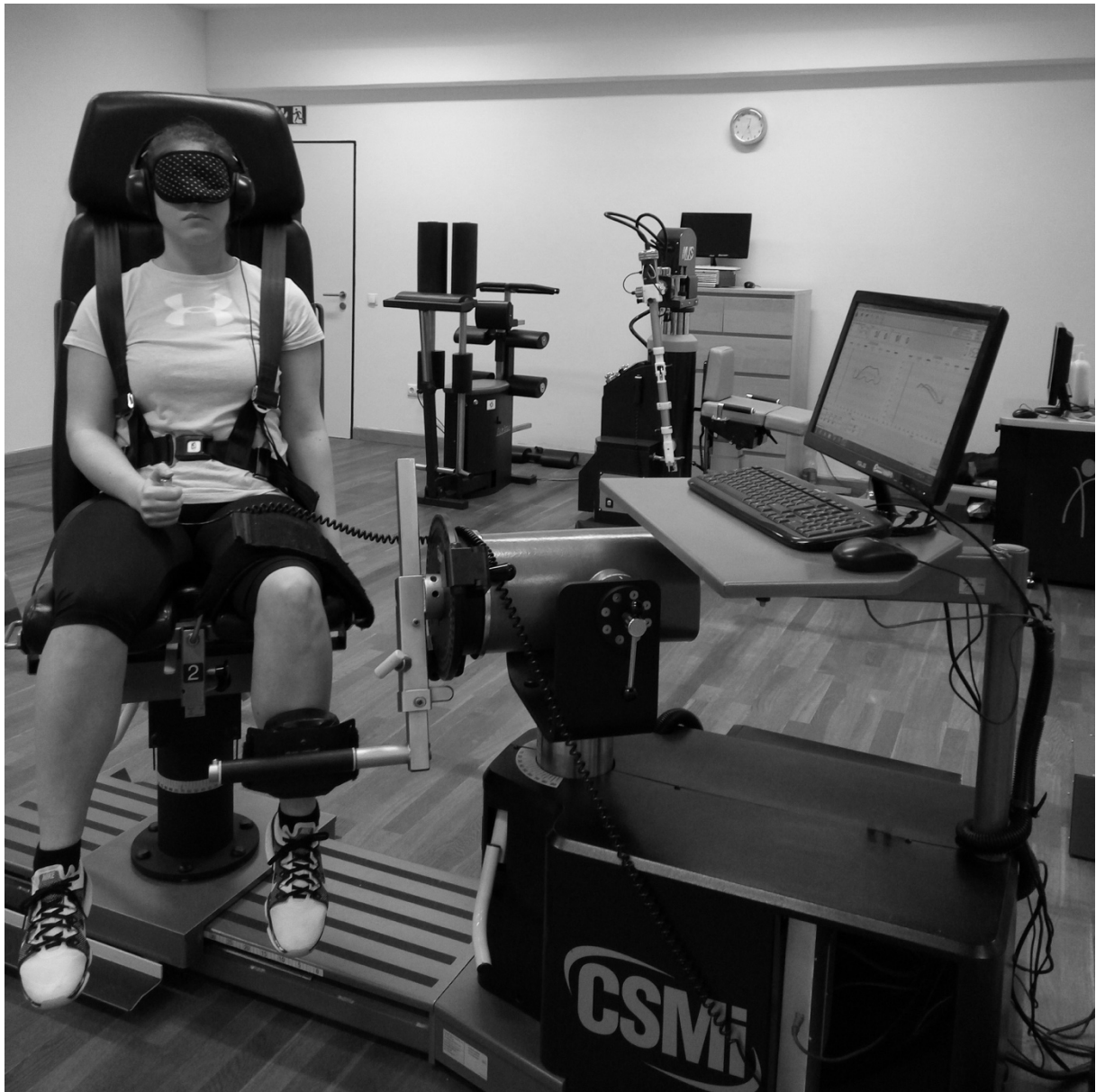
Fig. 1. Set-up for the proprioception measurements (Galamb et al. 18). Participants were seated in the dynamometer chair in an upright position. One leg hanged freely over the edge of the chair and the other leg was fixed to the attached free-moving arm, with a flexion angle of approximately 90^\circ . Subjects wore blindfolds for both tasks to eliminate vision and headphones with white noise in the motion sense task to eliminate auditory cues.
