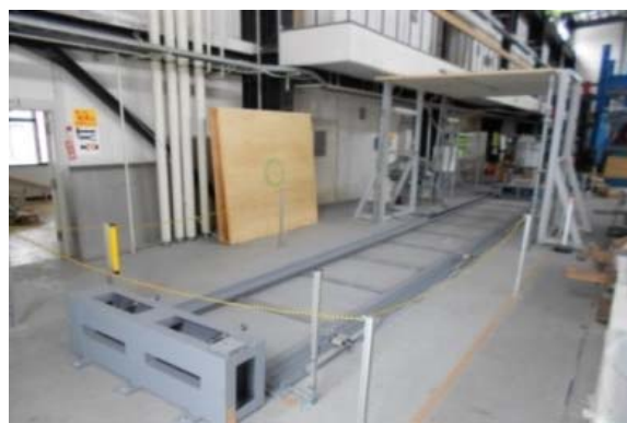
(b) Rails on which the blower moves
