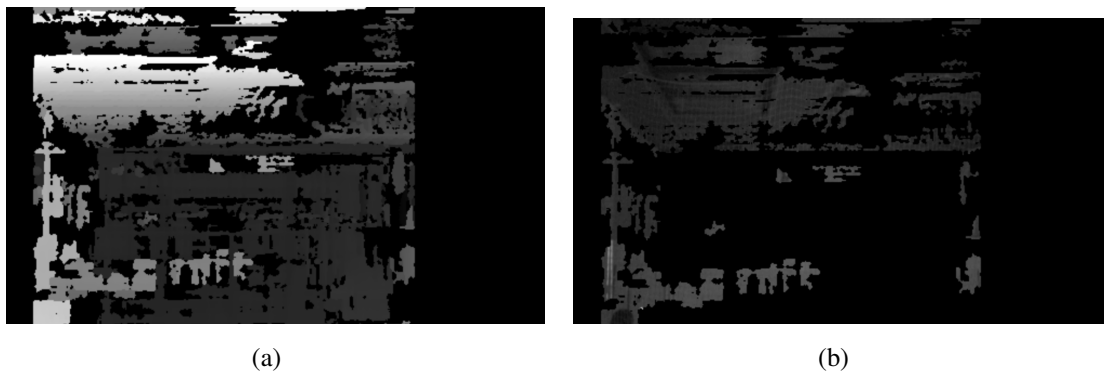
Figure 2.7: Disparity map obtained using semi-global block matching algorithm [1] (a) and superposition top half of disparities on the corresponding image (b)
