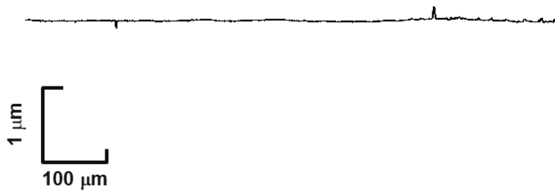
(b) Wear track on SiC disk
