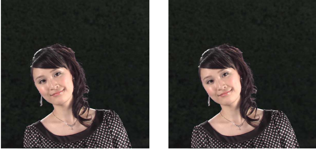
(a) Target picture predicted with a translation for each block (b) Target picture predicted with two translations for split blocks
