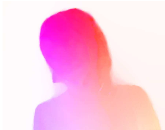
(c) Visualization of the optical flow between 4.1a and 4.1b. Color intensity shows absolute value of the motion vector and tint the direction
