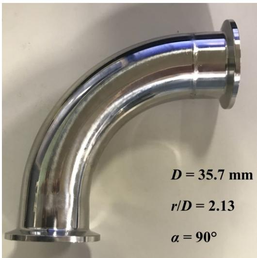
**Fig. 3-24** Bend 4C and its dimensional parameters.
