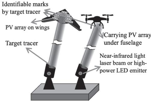
Figure 1 Feeding or charging in-flight drone through OWPT
