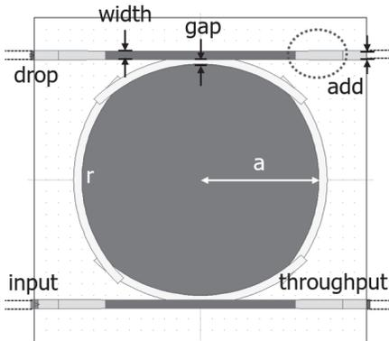
Figure 2 The basic structure of the filter
