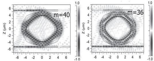
Figure 3 Different propagation modes at different wavelengths
