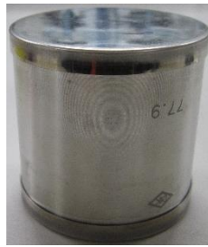
Fig. 2-17 Mold for permeability test
