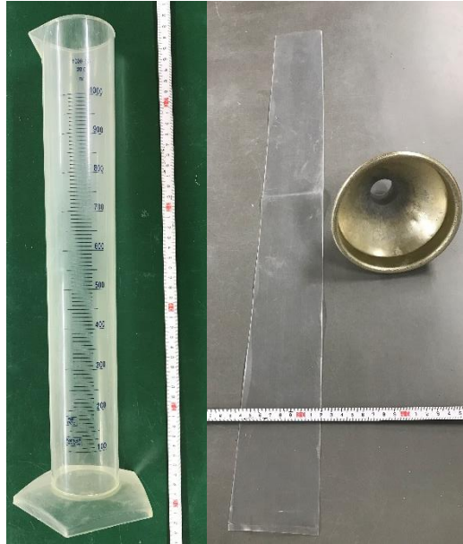
Fig. 3-3 Tools of bleeding test
