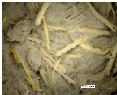
Fig. 3-21 Microscope image of fiber-reinforced cemented soil
