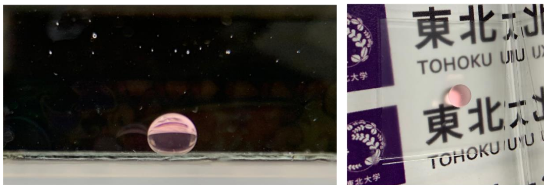
Figure 2-17. Oil droplet on the 5PC60 underwater and the image on a piece of paper.
