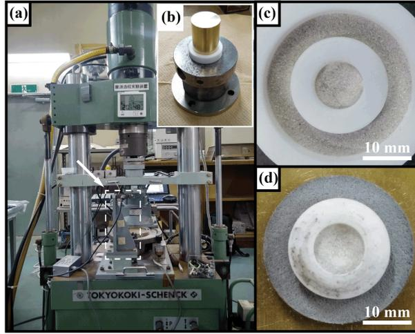
**Fig. 2:** The overall view of a low-velocity rotary shear apparatus and simulated-quartz gouge before and after shear tests (Tanaka et al., 2021). (a) A low-velocity rotary shear apparatus. A white arrow points a torque arm. (b) A part of an assembly to set in the apparatus. (c) Starting and (d) sheared quartz gouges on the surface of the brass forcing blocks. Note the color change of gouge after a shear test in (d).
