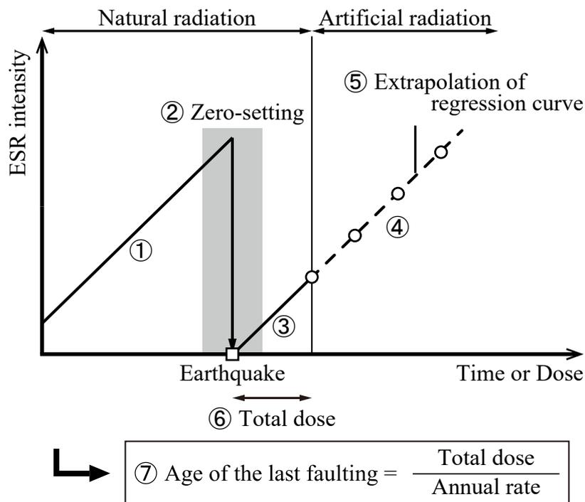
Fig. 1: The principle of fault dating using ESR (Tanaka et al., 2020).
