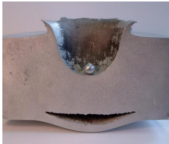
Fig. 1.3: Damage caused by a small sphere of aluminum to a block of 18 cm thick aluminum at hyper velocity. (©ESA)
