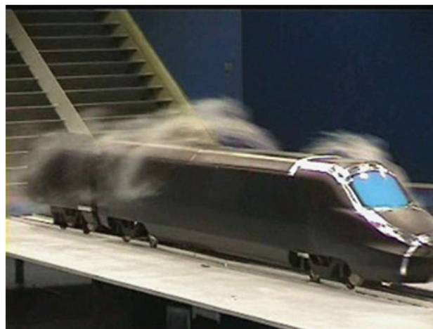
Figure 1.4 Crosswind wind tunnel test described in the EN (Bocciolone et al., 2008)
