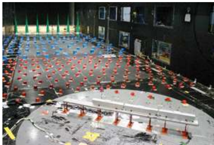
Figure 1.3 Wind tunnel test simulating natural crosswind (Kikuchi and Suzuki, 2015)
