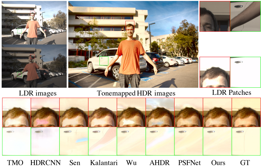
Figure 3.8: Results from the Testing data (08) of [1]. Upper row from left to right: the two input LDR images, the HDR image produced by the proposed method, and (zoomed-in) LDR image patches with two identical positions/sizes (in green and red). Lower row: the same patches of the HDR images produced by different existing methods
