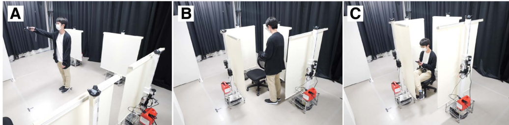
Figure 7: Ad hoc private spot builder: A) A user designs the partitions' layout. B) The system creates the designed layout. C) A private spot is configured using four partitions.
