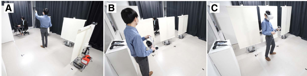
Figure 12: Ad hoc physical shielder: A) A user enters the room where another user is already working, and he starts arranging partitions. B) The configured partitions separate the room. C) While the HMD-wearing user performs VR interactions with full-body gestures, each user can safely concentrate on his task without the risk of collision.
