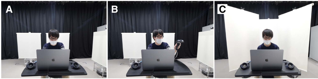
Figure 8: Meeting booth creator: A) A user focuses on a personal task at his desk. B) He invokes a preset layout before starting an online meeting. C) He gets a neutral white background that protects his monitor from "shoulder surfing."
