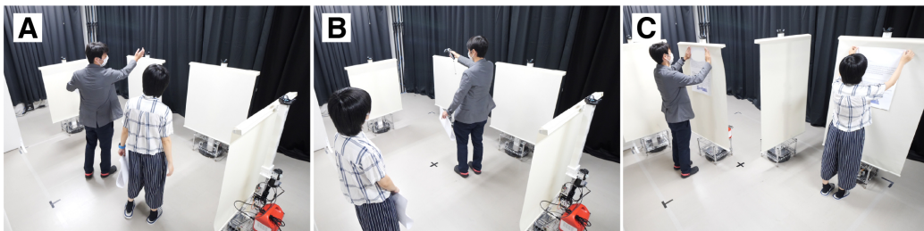
Figure 11: Exhibition layout editor: A) Two presenters discuss the presentation layout in an exhibition hall. B) A man arranges the partitions with the controller. C) The partitions form the poster booth layout, and presenters attach their posters to the partitions.
