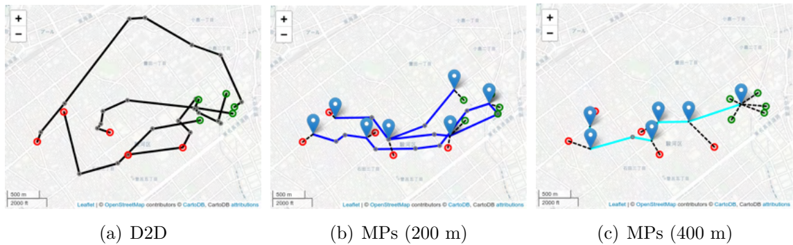
Figure 6.16: Examples of D2D-based and MPs-based OSMS routes. The green circle indicates the origin and the red circle indicates the destination. The gray circles indicate the pick-up/drop-off points of the demand handled by the vehicle in addition to the five ODs. The light blue markers are MPs. The black solid lines indicate vehicle trajectories and the dotted lines indicate passenger walkways.
