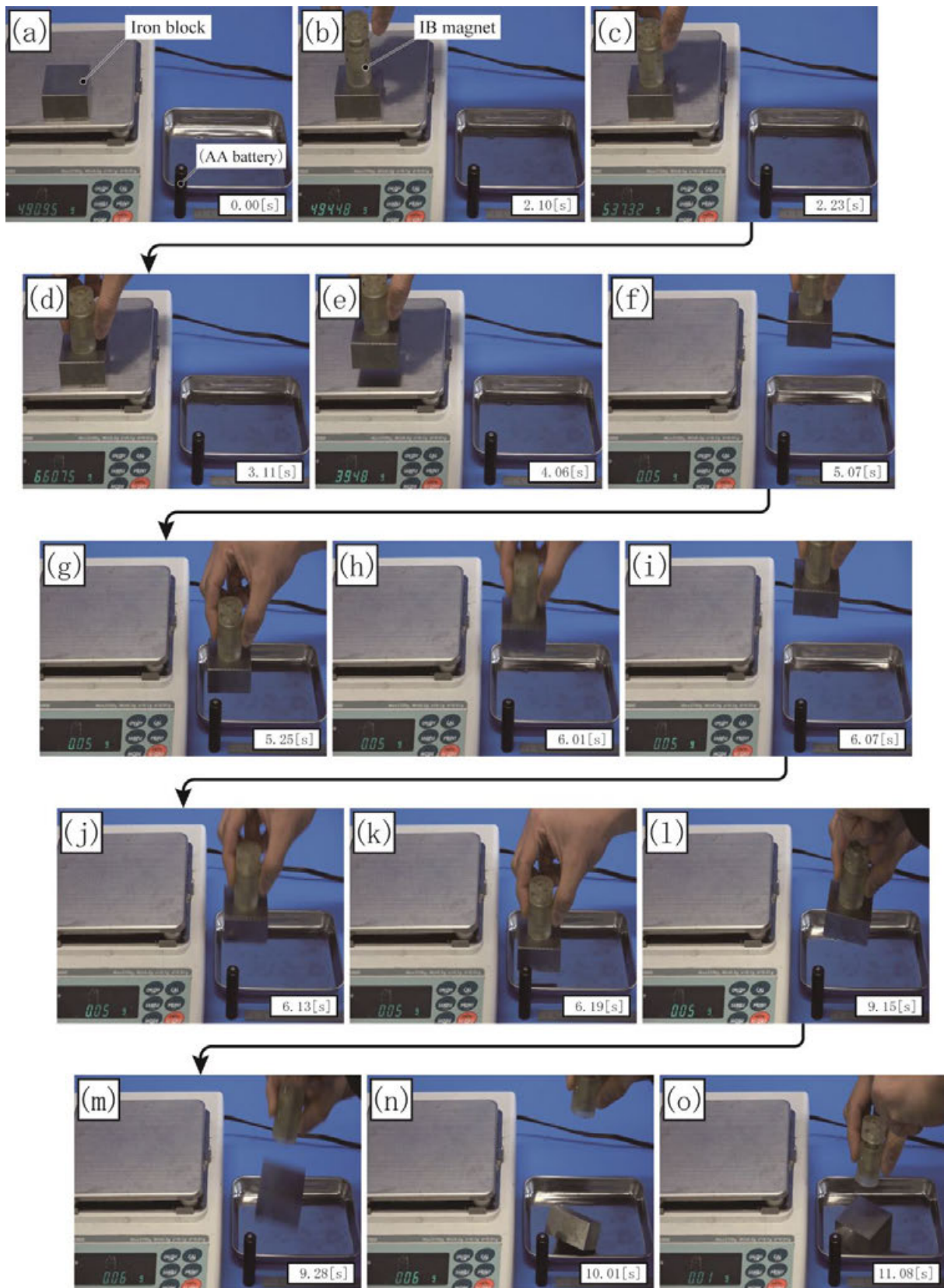
Fig. 72 Basic operation of the prototype of the IB magnet using the magnetic spring.
