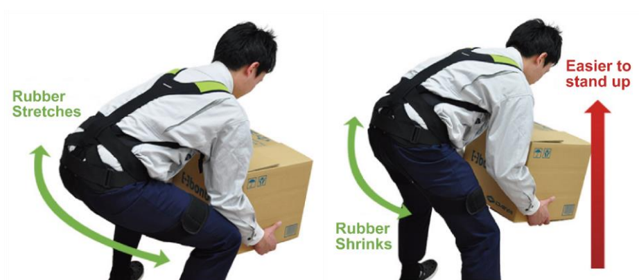
Fig. 10 Assistive function of an unpowered assistive suit, whose elastic rubber on the buttocks generates a tension force to the support user to life a heavy load [26].
