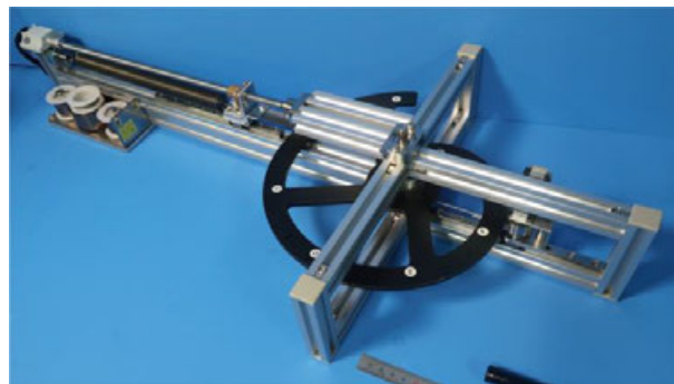
Fig. 15 Appearance of the POC model of the proposed displacement–force converter using the pressure angle method.
