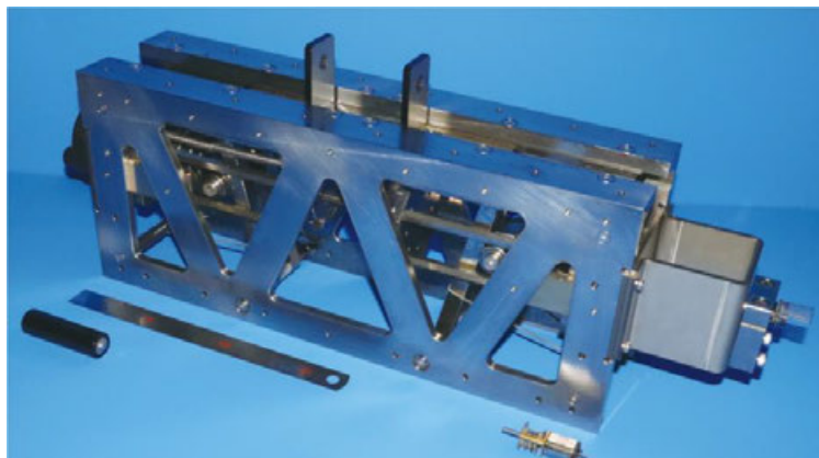
Fig. 97 Appearance of the prototype of the bi-parting IB magnet using the magnetic spring with the adjustable clamping width.
