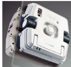
Fig. 58 A pair of window-cleaning robots with a magnetic distance adjustable by a screw [61].
