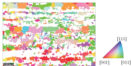
Fig.1 Inverse pole figure map of bcc in a duplex iron alloy against RD and stereo triangle.
