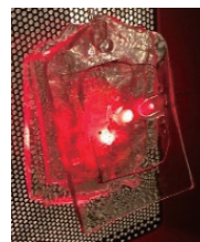
(b) Experiment using C-shaped loop type rectenna array
