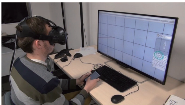
Figure1: In-VR text typing interface using smartphone touch screen with confirm-on-release paradigm (visual cues)
