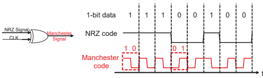
Figure 2: Waveforms of NRZ and Manchester code
