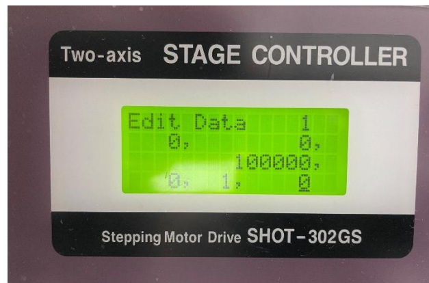
Fig. 6.10. Front panel of two-axis stage controller illustrates the editable program.
