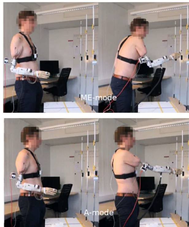
Figure 1.12: The experimental setup in [64] for reaching movements with initial and final postures towards the target with the ME-mode ( myoelectric control) and with the A-mode (automatic elbow control).
