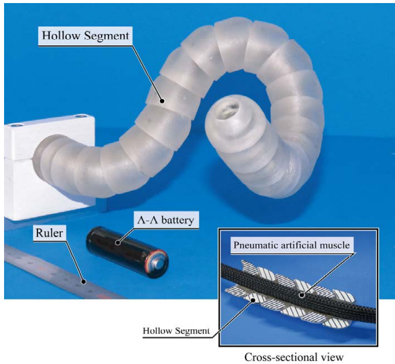
Fig. 56 Prototype of the proposed variable stiffness mechanism consisting of a pneumatic artificial muscle enclosed in a link structure.
