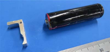
Fig. 47 Levers for wire cramping. The outer radius of the spherical surface where the lever contacts the rubber tube is 7.0 mm.
