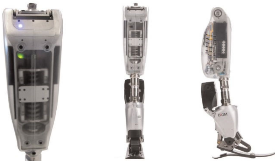
Fig. 7 Clutchable series-elastic actuator knee using electromagnetic brake [42].
