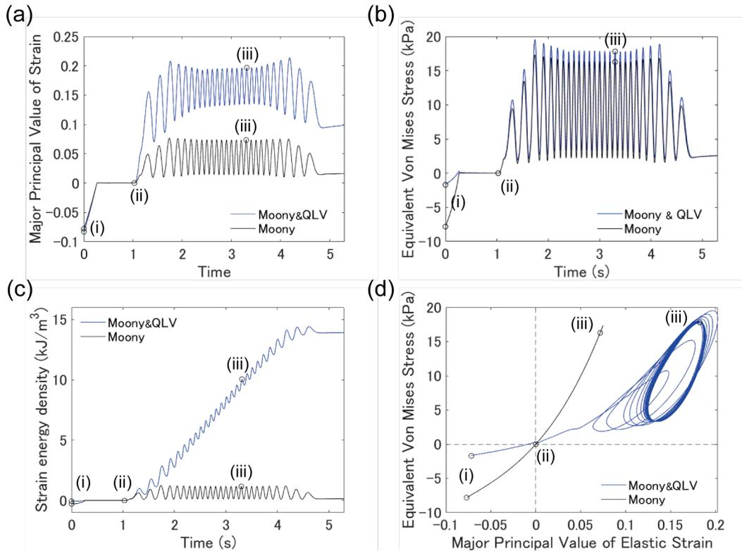
FIGURE 4.8: SED accumulation induced by periodic stimulation occurs due to viscoelastic effect.
