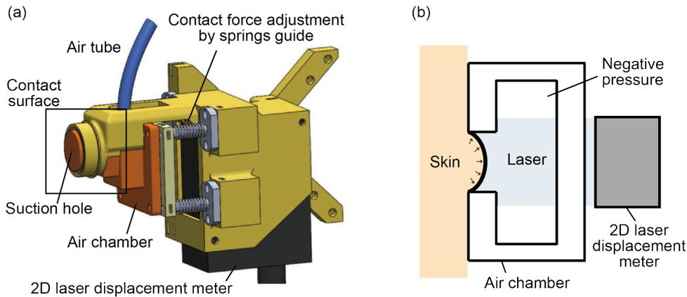
FIGURE 4.1: Configuration of a contactor of the developed suction device.
