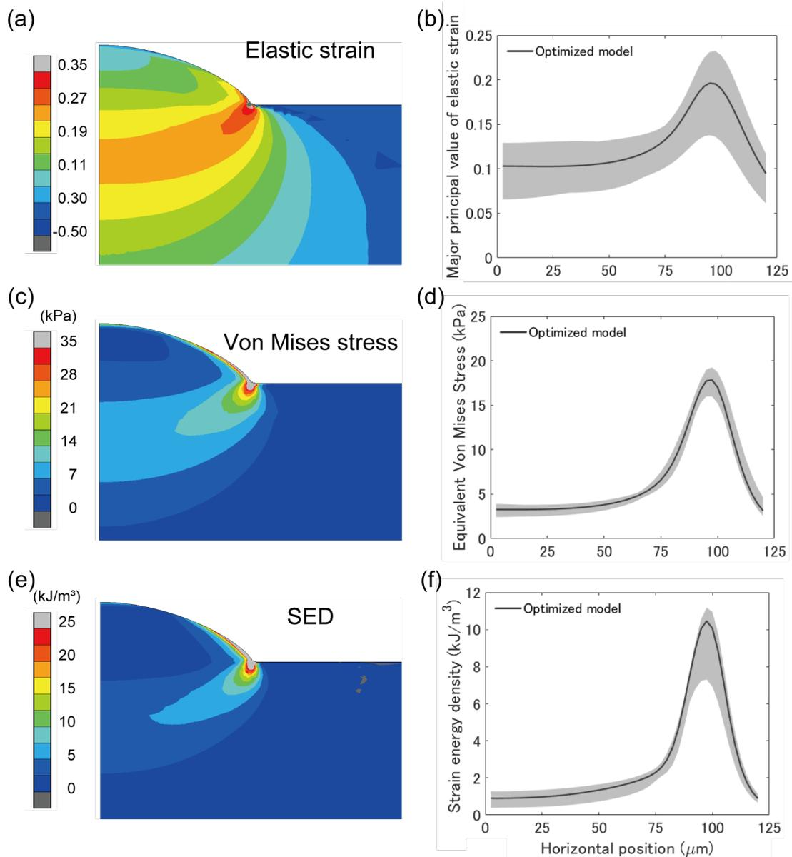
FIGURE 4.6: Simulated effect on how changes to skin material properties influence the interior mechanical quantities propagation.
