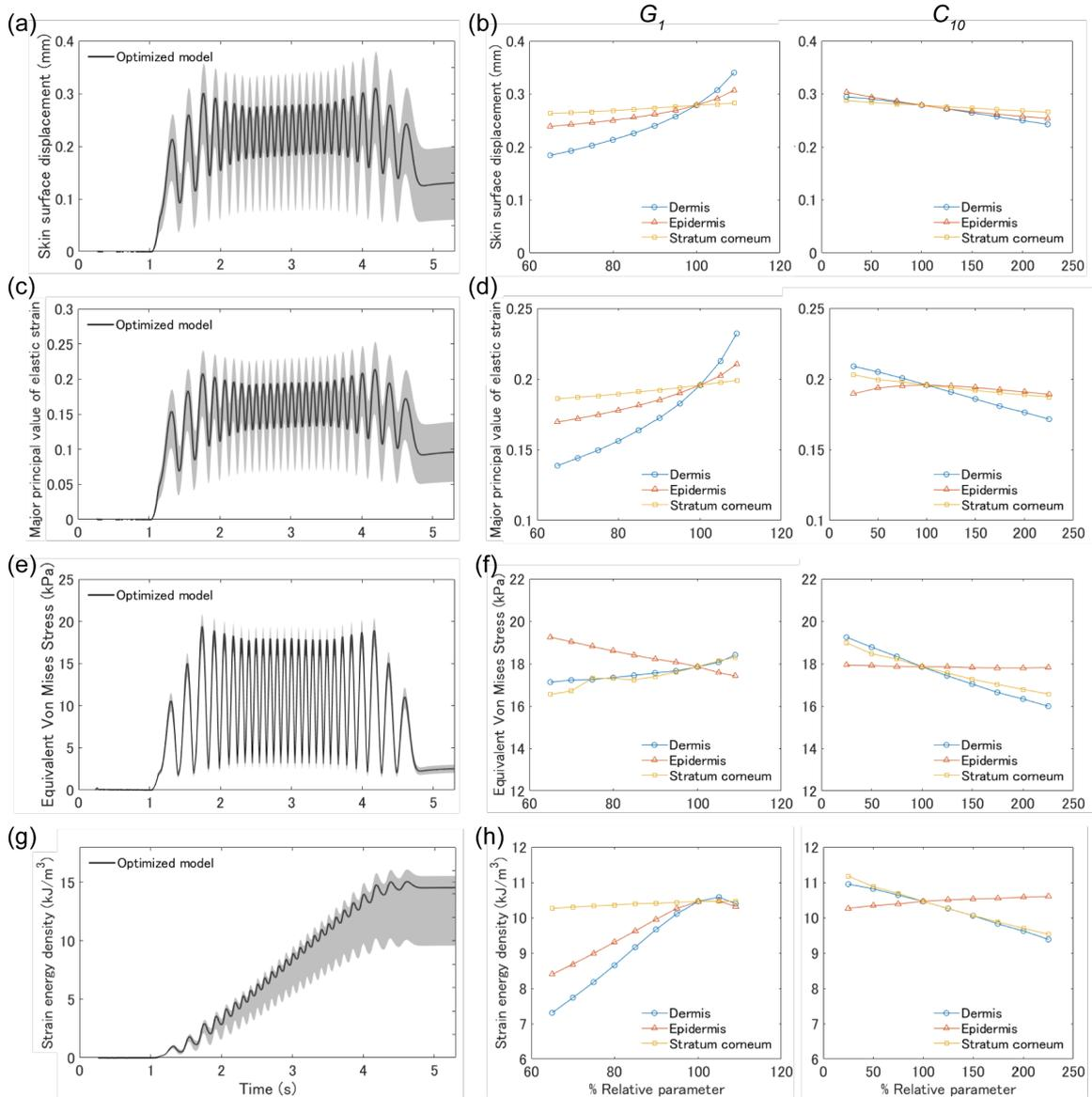
FIGURE 4.7: Simulated effect on how changes to skin material properties influence the interior mechanical quantities propagation.
