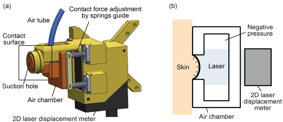
FIGURE 3.1: Configuration of a contactor of the developed suction device.
