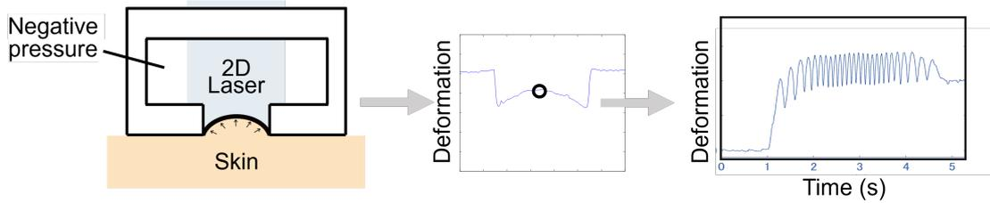
FIGURE 2.4: The method for obtaining skin deformation.
