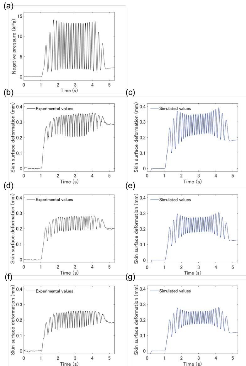
FIGURE 4.5: Comparison of the experimental data and numerical simulation based on the optimized material parameters.
