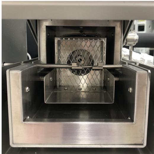
FIGURE 3.7: Photograph of the dynamic elastic modulus measuring apparatus.
