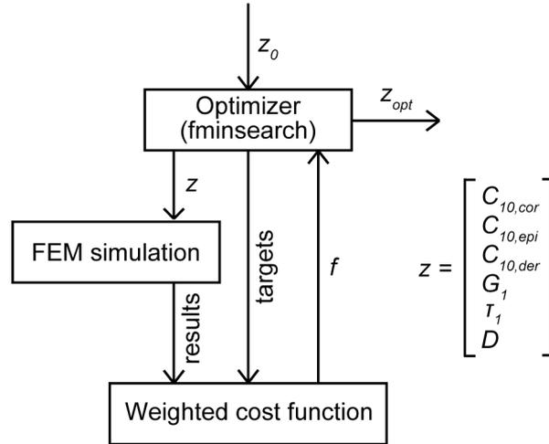
FIGURE 4.3: Schematic representation of the optimization scheme for the material parameter identification.
