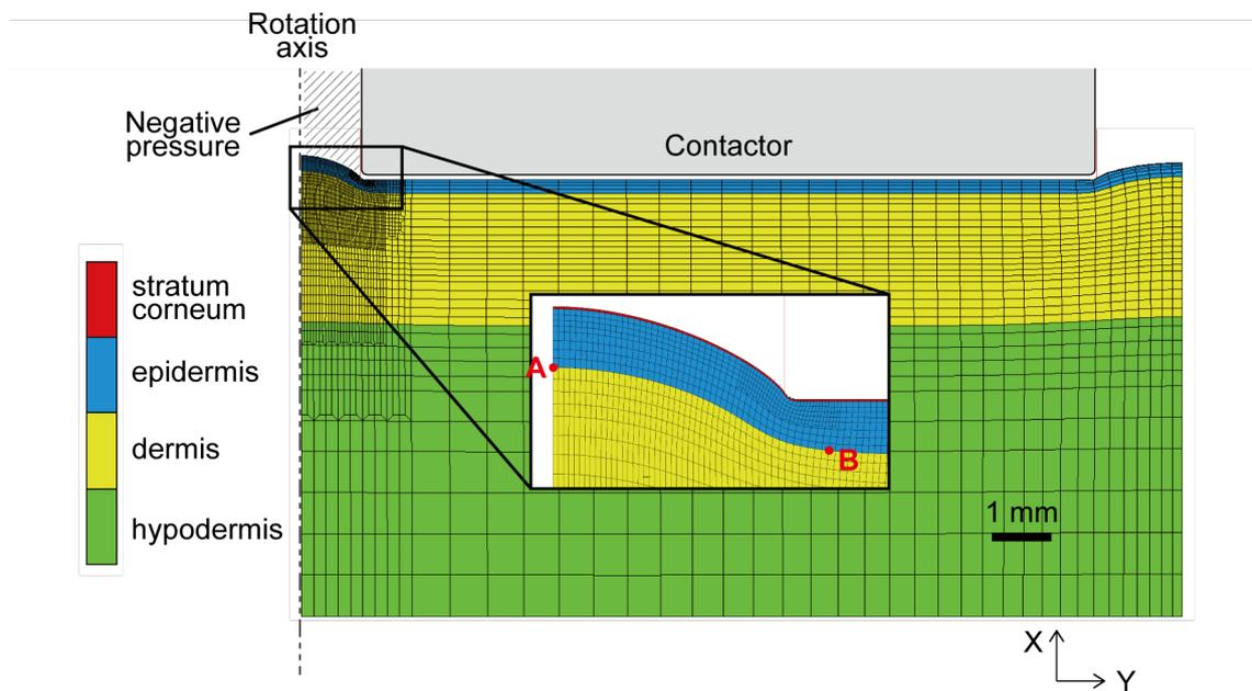
FIGURE 4.2: Illustration of the finite element (FE) model used in the analysis.
