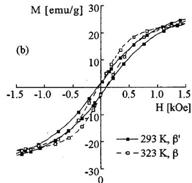
FIG. 3. Magnetic properties of the  $Ni_{33.5}Co_{38.5}Al_{28}$  FSMAs. (a)  $M-T$  curve in an external magnetic field of 500 Oe. (b)  $M-H$  curves at 293 and 323 K upon heating. Note that the stable phase is  $\beta'$  at 293 K and  $\beta$  at 323 K.
