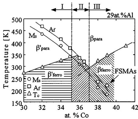
FIG. 1. Composition dependence of the Curie temperature  $T_C$ , the martensitic transformation temperature  $M_s$  and the austenitic finishing temperature  $A_f$  in  $Ni_{71-x}Co_xAl_{29}$  alloys. The FSME can be observed in the hatched region.
