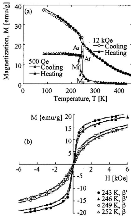
FIG. 4. Magnetic properties of the  $\text{Ni}_{35}\text{Co}_{35}\text{Al}_{30}$  alloy. (a)  $M$ - $T$  curves in external magnetic fields of 500 and 12 000 Oe. (b)  $M$ - $H$  curves at 243, 246, 249, and 252 K upon heating. Note that the stable phase is  $\beta'$  at 243 and 246 K and  $\beta$  at 249 and 252 K.
