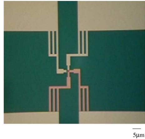
Fig. 2. Top view of the via Kelvin pattern after CMP by optical microscopy.
