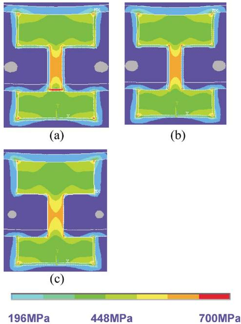
Fig. 11. Simulated stress distribution of Cu dual-damascene interconnects. (a) 15-nm thick barrier layer on the bottom and sidewall of the via and trench. (b) No barrier at the via bottom. The thickness of barrier layer except via bottom is 15 nm. (c) No barrier at the via bottom, either. The thickness of barrier layer except via bottom is 2 nm.
