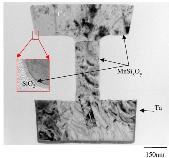
Fig. 3. Cross-sectional TEM images of Cu dual-damascene interconnects with self-formed  $\text{MnSi}_x\text{O}_y$  barrier layer.
