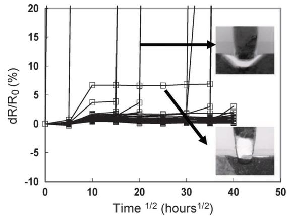
Fig. 9. Relative resistance-increase behavior of PVD Ta samples as a function of square root of the testing time, including cross-sectional TEM images of the SiV pattern after SiV testing.
