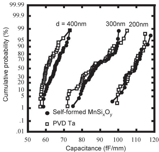
Fig. 7. Distribution of capacitance at intralevel. Spaces were 200, 300, and 400 nm.
