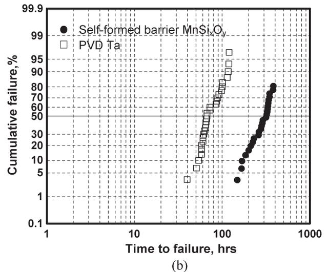
Fig. 12. EM cumulative failure distribution of PVD Ta and self-formed  $\text{MnSi}_x\text{O}_y$  barrier samples. Electron-flow direction of (a) and (b) are from M1 lower line through the via to M2 upper line and M2 line through the via to M1 line, respectively.
