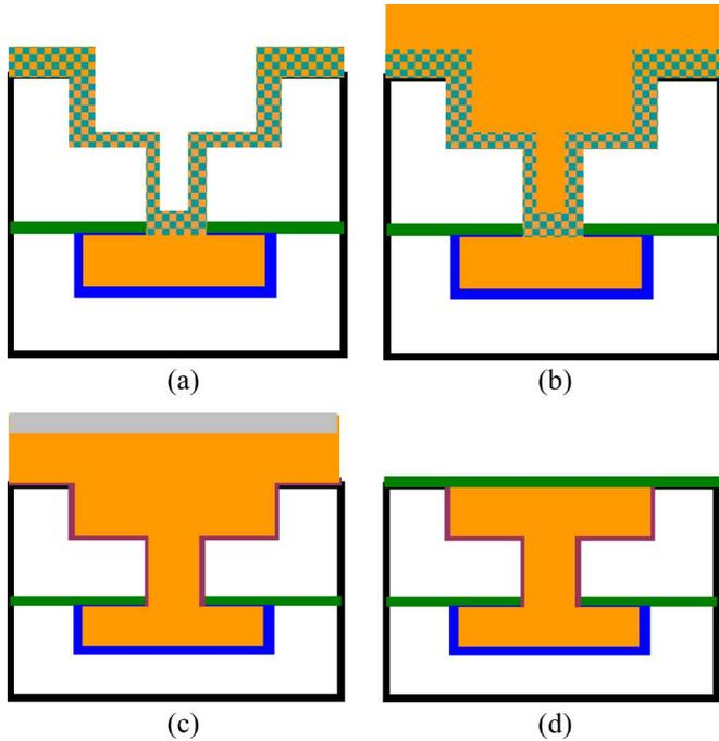
Fig. 1. Schematics of the fabrication process for Cu dual-damascene interconnects with self-formed  $\text{MnSi}_x\text{O}_y$  barrier layer. (a) Deposition of CuMn seed layer by sputtering. (b) Cu deposition by electrochemical plating. (c) Annealing for  $\text{MnSi}_x\text{O}_y$  layer. (d) Removal of excess Cu and Mn by CMP and deposition of dielectric diffusion barrier.
