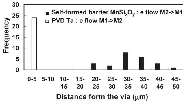
Fig. 13. Distribution of EM-induced void location of PVD Ta and self-formed MnSi<sub>x</sub>O<sub>y</sub> barrier samples.
