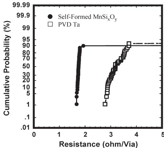
Fig. 8. Distribution of via resistance. Number of the vias is 100 000 and via diameter is 140 nm.
