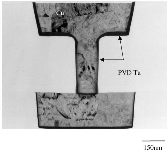
Fig. 4. Cross-sectional TEM image of Cu dual-damascene interconnects with conventional PVD Ta.
