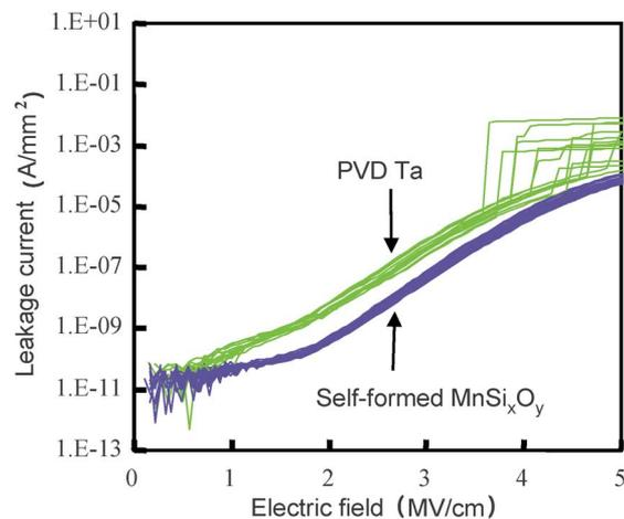
Fig. 6. Leakage current as a function of applied electrical field.
