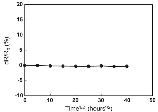
Fig. 10. Relative resistance-increase behavior of self-formed  $\text{MnSi}_x\text{O}_y$  barrier samples as a function of square root of the testing time.
