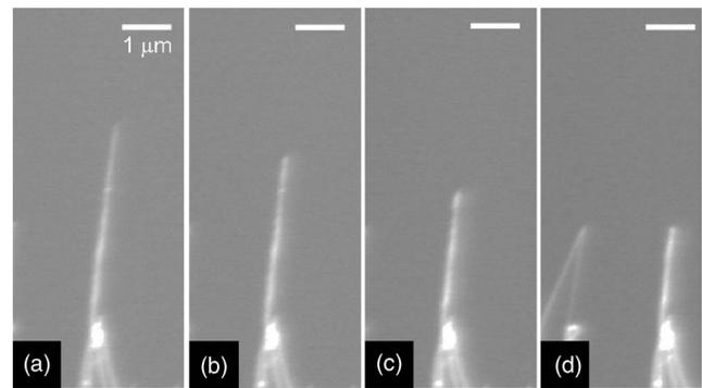
FIG. 3. (a) Before and [(b)–(d)] after cutting of a single CNT in less than 1 min. (b) A length of 650 nm was cut off the first time, (c) a further 700 nm was cut off the second time. (d) The CNT on the right after cutting has the same length as the one on the left.
