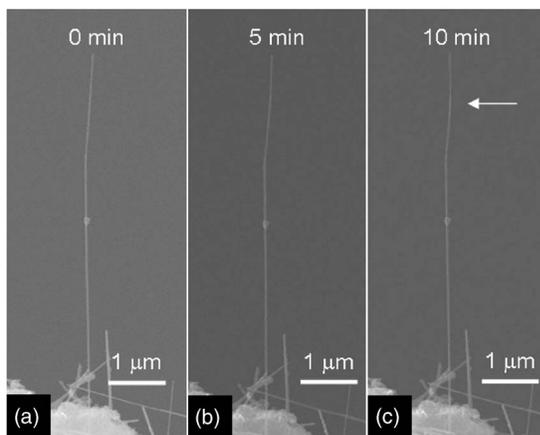
FIG. 2. Single CNT exposed to an electron beam with the introduction of oxygen gas. In this case, the nozzle is far from the cutting object. The results of irradiation after (a) 0 min, (b) 5 min, and (c) 10 min are shown.
