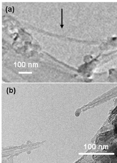
FIG. 5. TEM images of MWCNTs (a) before and (b) after cutting. It was estimated that about 100 nm of material was removed.
