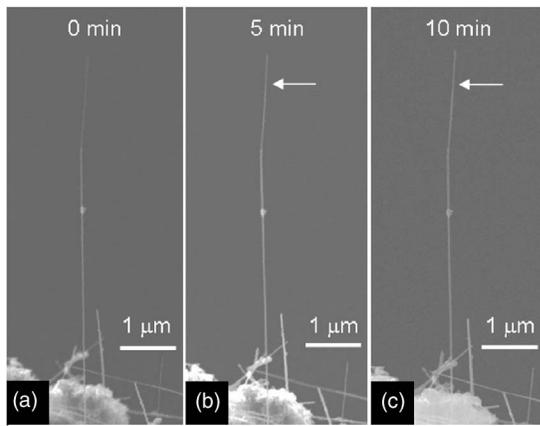
FIG. 1. Single CNT exposed to an electron beam without the presence of oxygen gas. No changes in the CNT were observed. The beam exposure times are (a) 0 min, (b) 5 min, and (c) 10 min.
