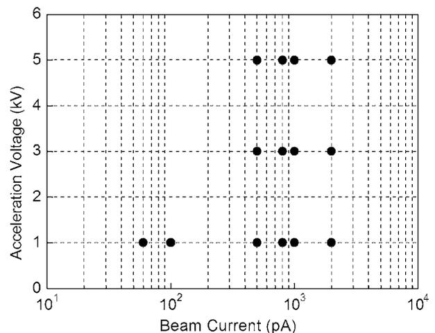
FIG. 4. Cutting of CNTs in less than 1 min under various acceleration voltages and beam currents shown by the black circles.
