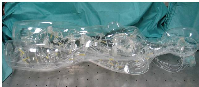
Fig. 16 Surgical Simulator for endovascular intervention, comprised of patient-specific vasculature model of whole human aorta structure
