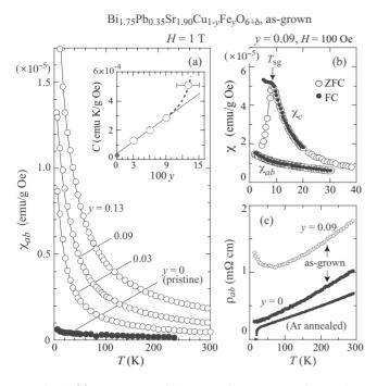
FIG. 1. (a)  $\chi_{ab}$  over a wide range of temperature for H=1 T. The inset shows C as a function of the Fe content. (b)  $\chi_{ab}$  and  $\chi_c$  at low temperatures for H=100 Oe and y=0.09. (c)  $\rho_{ab}$  for y=0.09 (as-grown) and y=0 (as-grown and Ar-annealed).
