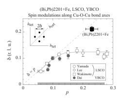
FIG. 5. Comparison of  $\delta$  between Fe-doped (Bi,Pb)2201, pristine La214 (Refs. 9, 16, and 17), and Y123 (Ref. 12). Dynamical data are plotted for La214 ( $\omega$ =3-6 meV at  $T \sim T_c$ ) and Y123 ( $\omega \ll$  (resonance energy) at  $T < T_c$ ). The *p* range of the superconducting phase is indicated by a thick bar at the base line. The solid line is a guide for La214 and Y123 data.
