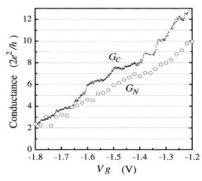
FIG. 4. The constriction conductance  $G_c$  measured at V = 0 and the conductance  $G_N$  measured at a high voltage are shown as a function of  $V_g$ .
