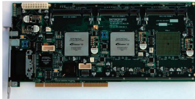
Fig. 6. DiNI group DN7000k10PCI with two Stratix II FPGAs (EP2S180).
